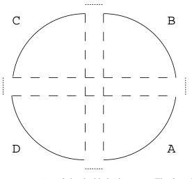
Fig. 4 Schematic representation of the double-bridge move. The four dotted edges are removed and the remaining parts A, B, C, D are reconnected by the dashed edges.
