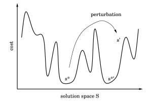
Fig. 2 Pictorial representation of iterated local search. Starting with a local minimum  $s^*$ , we apply a perturbation leading to a solution s'. After applying LocalSearch, we find a new local minimum  $s^{*'}$  that may be better than  $s^*$ .
